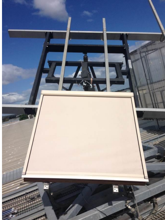
Test Window with screen closed on Solar Test Stand.
