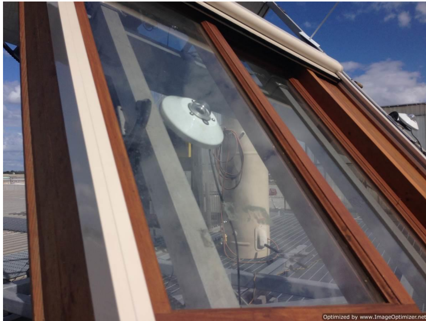
Solar Pyranometer behind Glass for test 1.
